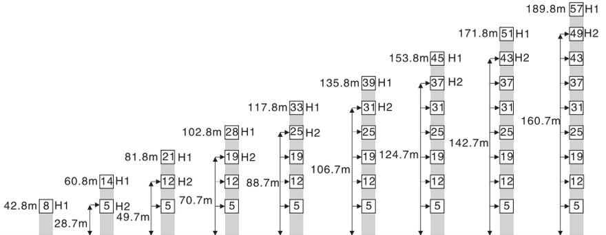
H1—臂根铰点下高度 Height under jib hinge shaft
